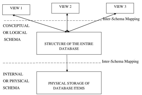
The word schema means arrangement – how we want to arrange things that we have to store. The diagram above shows the three different schemas used in DBMS, seen from different levels of abstraction.
